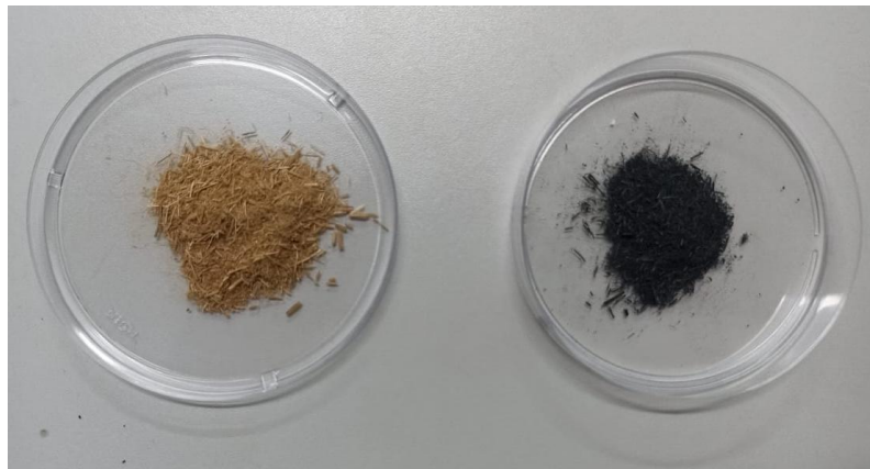
Figure 10 - Conversion of biomass to biochar - (a) Raw Petiole and (b) Petiole Biochar.
