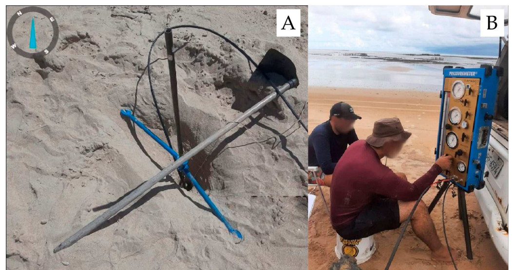
Figure 6. (A) Borehole for pressuremeter test and (B) test execution.
