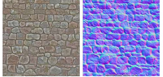
Fig. 3: On the left: stone wall texture, on the right: its corresponding normal map texture. (Source: docs.unity3d.com)
