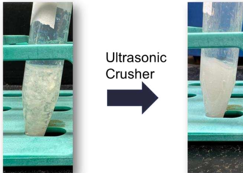
Figure 38 – Illustrations of the BCF suspension in NSC solution before and after the ultrasonic crush process
