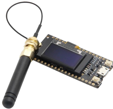
Figura 12 – TTGO LoRa32 SX1276 OLED
