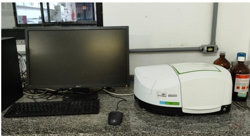
Figura 18 – Espectrômetro Perkin-Elmer Spectrum-Two.
