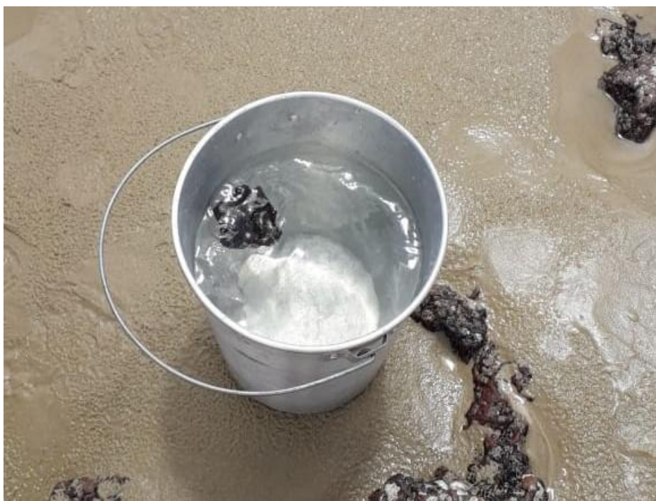
Fig. S2. Test of fluctuation of the waxy tarball, collected in late 2022 at the State of Ceará, Brazil, on sea water.
