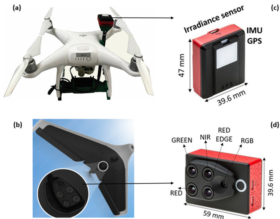
Figure 2. Depiction of the Sequoia (c,d) camera affixed to the Parrot Disco Pro AG (b) and DJI Phantom 4 (a) UAVs, facilitated by the utilization of a bracket and 3D printing. Source: Parrot 2020.
