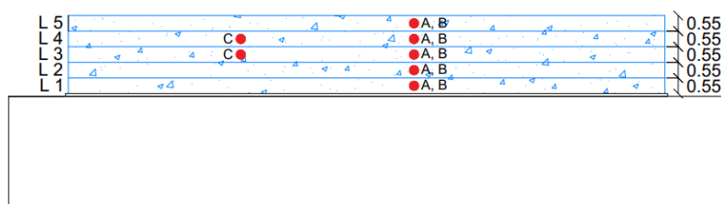
Figure 71 – Cross-section BB of the rafter with the location of points A, B, and C within the structure
