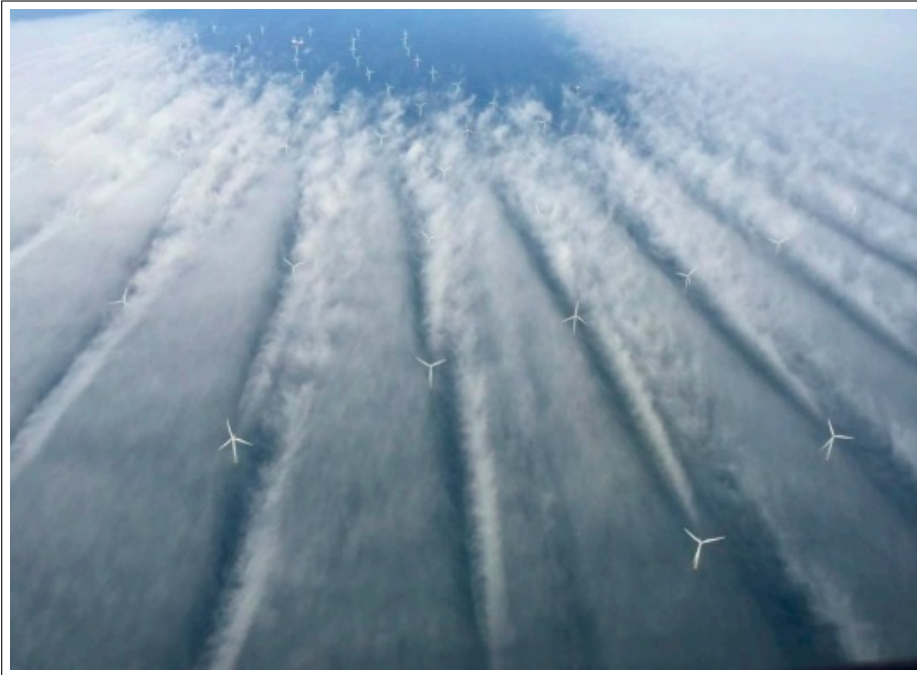
Figura 2 – Photos of wake effect captured in an offshore wind farm. Generation is higher in turbines with little intervention coming from its neighborhood
