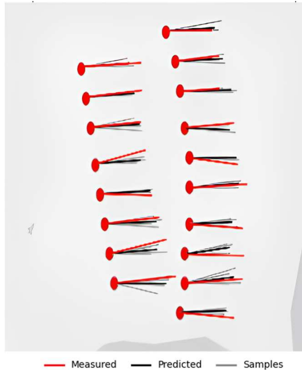
Figura 20 – Wind speed forecasts for each turbine in red, compared to ground truth ones in black. In light grey, samples yielded from the predictive distribution. Example extracted from ConvLSTM neural network, along with Deep Ensembles Bayesian framework.
