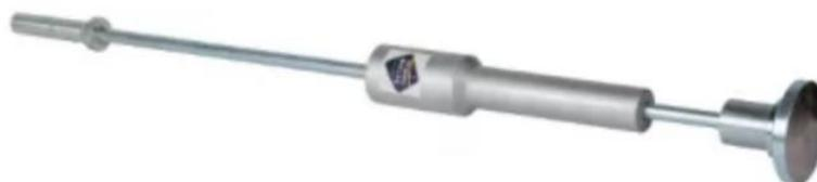
Figura 3 – Equipamento W.T.A.T (*Wet Track Abrasion Test*)
