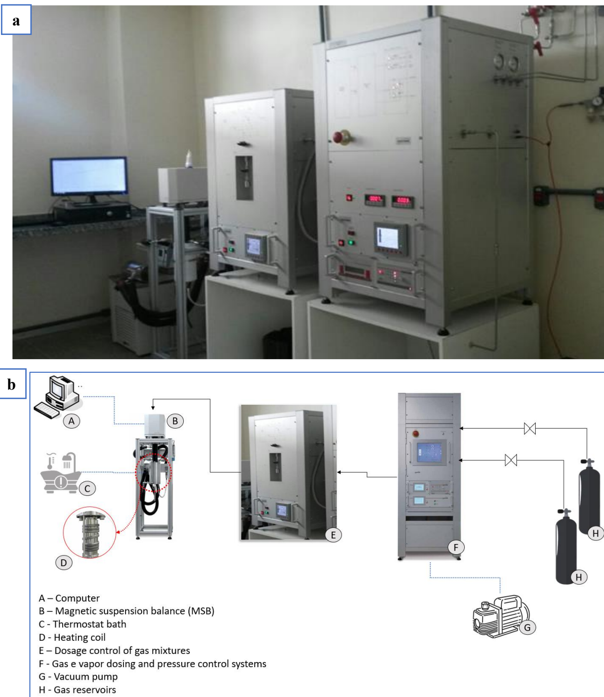
Figure 12 – (a) Magnetic suspension balance (MSB) components and (b) experimental setup
