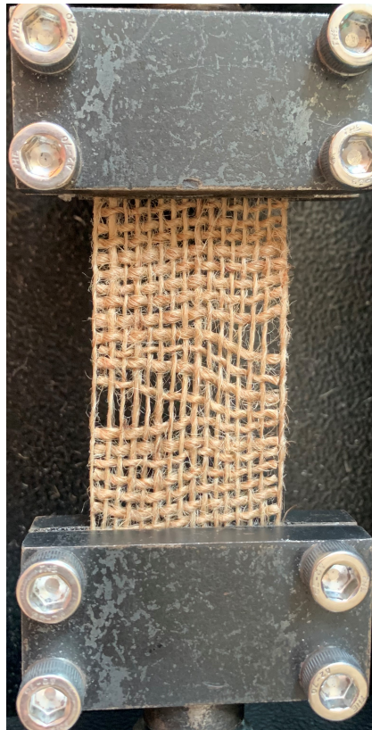
Figure 49 – Treated jute specimen after tensile test
