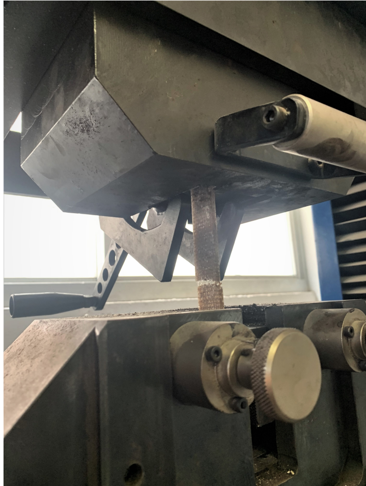
Figure 10 – Specimen after failure in the tensile test in the UTM.
