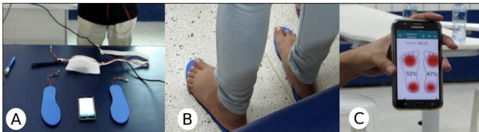
Figure 1: Development of the baropodometric insole prototype. A) Baropodometric insole prototype; B) Static position to determine the limit of symmetry between the affected and unaffected hemibody; C) Mobile health application developed to diagnosis and monitoring weight-bearing asymmetry.
