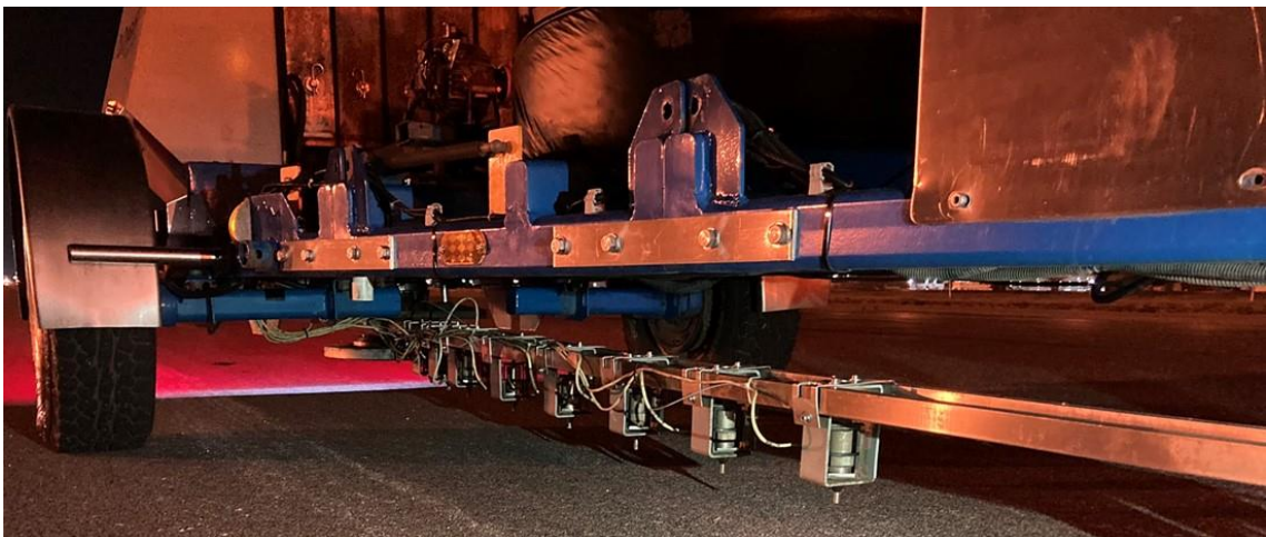
Figure 10 – Sensors used to measure the deflection basin and the plate load of FWD and HWD devices
