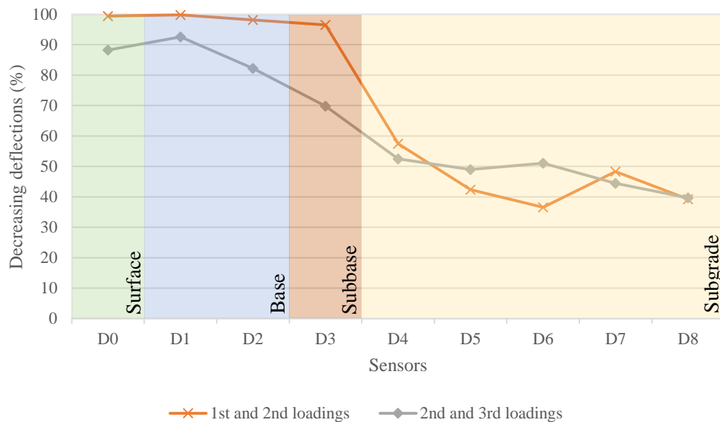
Figure 12 – Percentage of normalized deflections decreasing between two consecutive applications of 80kN-loads (Airport C)
