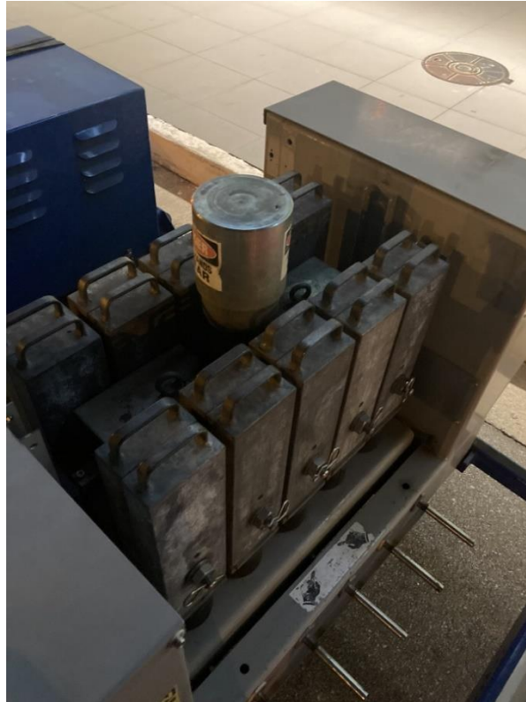
Figure 9 – The system of load application of FWD and HWD devices
