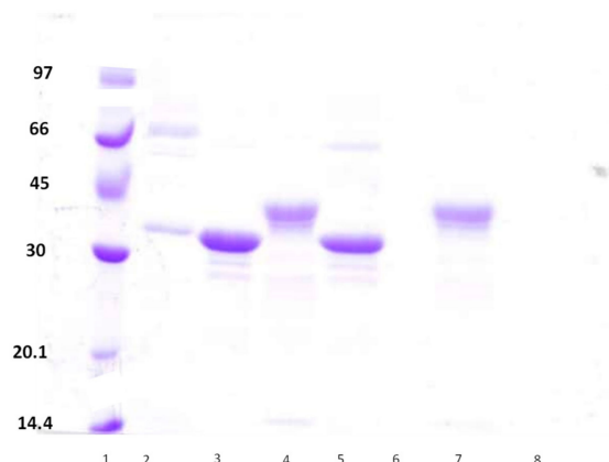
Figure 8. SDS-page analysis of combi-biocatalysts PFL-RML/PFL-LU. Lane 1: molecular weight marker, Lane 2: octyl-PFL; Lane 3: octyl-RML; Lane 4: octyl-LU; Lane 5: COMBI-PFL-RML; Lane 6: COMBI-PFL-RML washed with triton 4%; Lane 7: COMBI-PFL-LU; and Lane 9: COMBI-PFL-LU washed with triton 4%. Experiments were performed as described in Methods.
