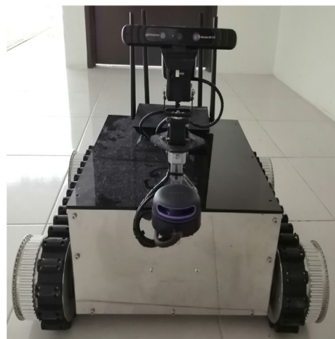
Fig. 4 Tracked robot equipped with Intel Real-sense depth camera and Lidar sensor
