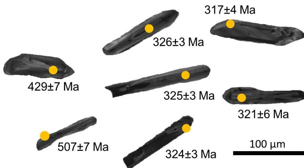
Figure 99 – Cathodoluminescence images of representative zircon grains from syn-D 2 granite dated in this study with ablation points and corresponding ages.
