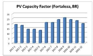
Fig. 4. Capacity factor data from a 1.5 kWp grid connected PV plant installed in Fortaleza, Brazil
