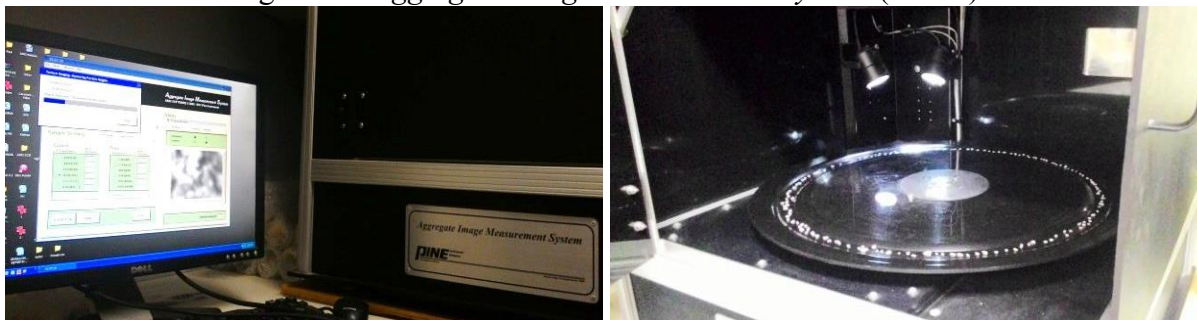
Figura 2 – Aggregate Image Measurement System (AIMS)
