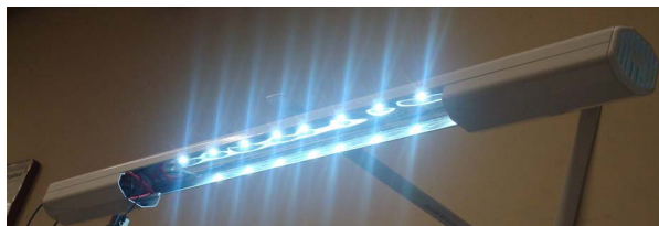
Figure 19. Lighting luminary with eight power LEDs.
