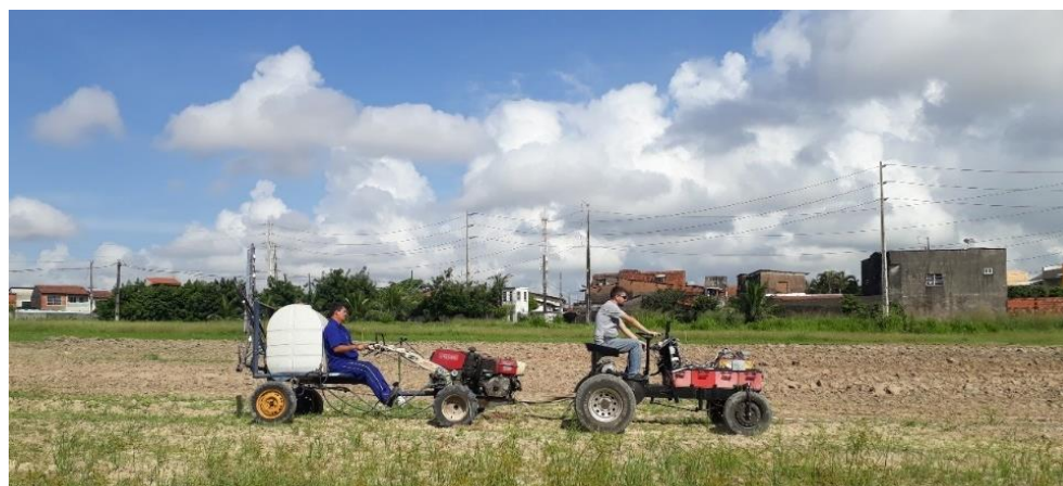
Figure 14. Electric tractor coupled to an agricultural sprayer and a 10.3-kW ICE tractor.
