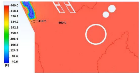
Figure 9. Temperature distribution with the solid ingot at 40° C 50% inserted into the zinc bath.
