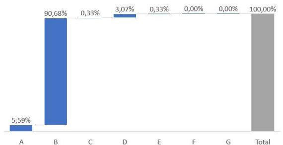
Figure 15. Destination of particles with ¼ ingot immersed (A= still in transit in the zinc bath; B= precipitated on the surface of the pot; C= precipitated on the surface of the internal snout bath; D= found the strip in the region 1; E= found the strip in region 2; F= found the strip in region 3; G= found the strip in region 4).
