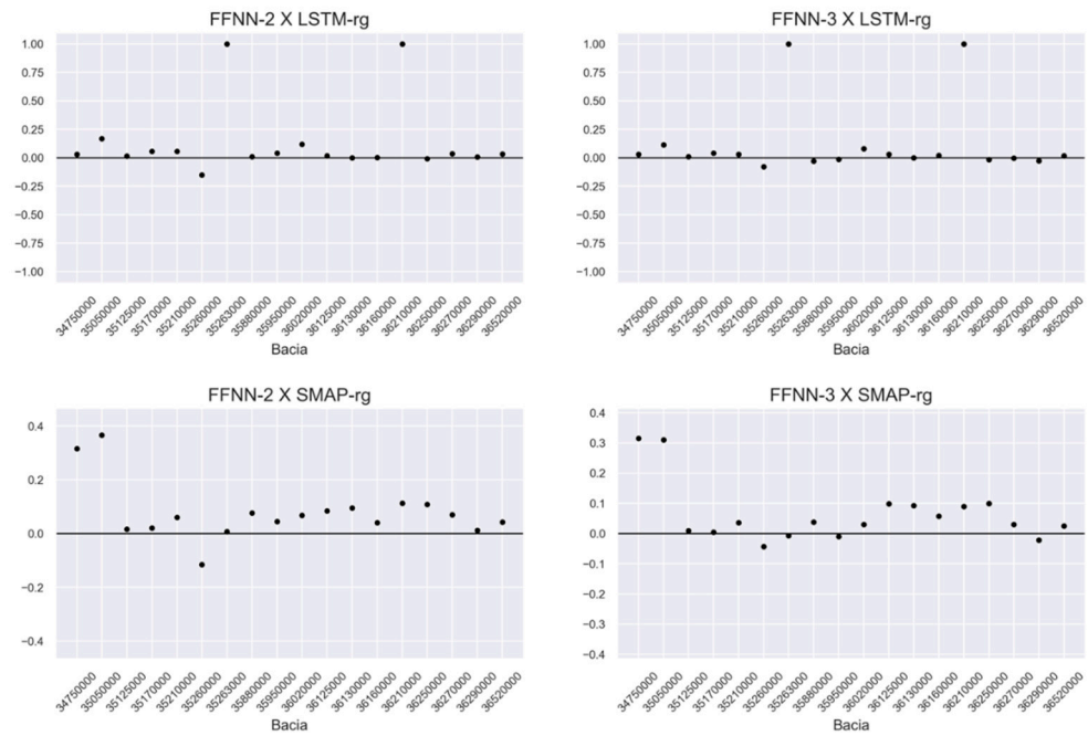
Figure 9. The y-axis represents the logarithm of the ratio of the NSE index of the FFNN-2 and FFNN-3 over the NSE index from the LSTM-rg and SMAP for all basins in the subset “iii” (x-axis).
