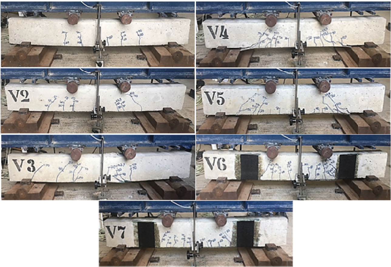
Figure 6. Beams after failure. Source: Author.
