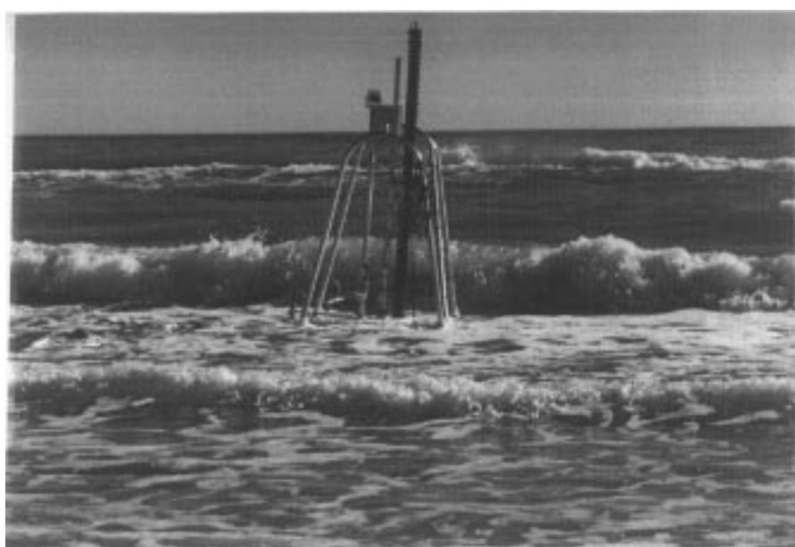
Instrumental sledge with 6 electromagnetic sensors, 1 wave gauge, 3 optical back scatters, 1 compass and 1 optical prism
