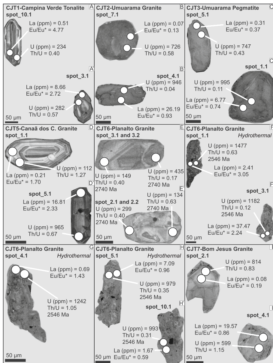
Fig. 5. SEM-Cathodoluminescence images of zircon crystals from analyzed samples from Carajás Province. (A) CJT1 – Campina Verde Tonalite has dominant magmatic zircon type (A), but some hydrothermal alteration is suggested by La enrichment and elevated Eu/Eu* (A'); (B) CJT2 – Umuarama Granite presents dominant hydrothermally altered zircon type, with elevated U contents and expressive variation of La contents (B and B'); (C) CJT3 – Umuarama Pegmatite presents the same geochemical behavior as CJT2 hydrothermally altered grains, with elevated U contents and variable La (C and C'), and both CJT2 and CJT3 present low variations on Eu/Eu*; (D) CJT5 – Canaã dos Carajás Granite is magmatic zircon, with preserved oscillatory zoning and regular U and La contents, and (D') is a hydrothermally altered crystal, with euhedral morphology and U and La enrichment and slightly high Eu/Eu*. (E) CJT6 – Planalto Granite magmatic zircon type (E) with low U contents and preserved oscillatory zoning. A zircon grain (E') present slight hydrothermal alteration, suggested by its massive texture. (F, G and H) CJT6 – Planalto Granite hydrothermal zircon type. These crystals present spongy texture, bread-crust texture (F, F' and H') diffuse rims (F, F', G, H and H'), and anhedral morphology and are enriched in U and La and present elevated Eu/Eu*. (I) CJT7 – Bom Jesus Granite zircons are magmatic (I) with slight hydrothermal alteration (I'), suggested by elevated La contents and massive texture.
