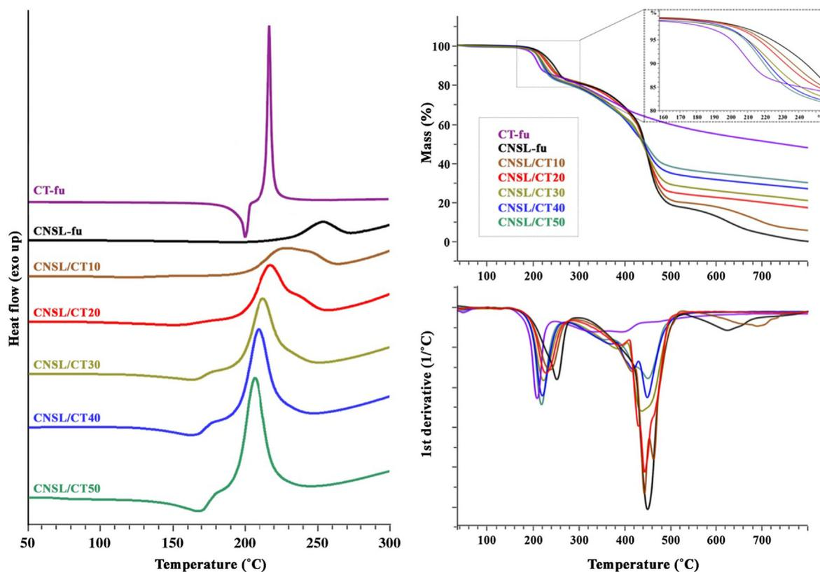
Fig. 3. DSC and TGA curves of CNSL-fu and CT-fu monomers and mixtures.
