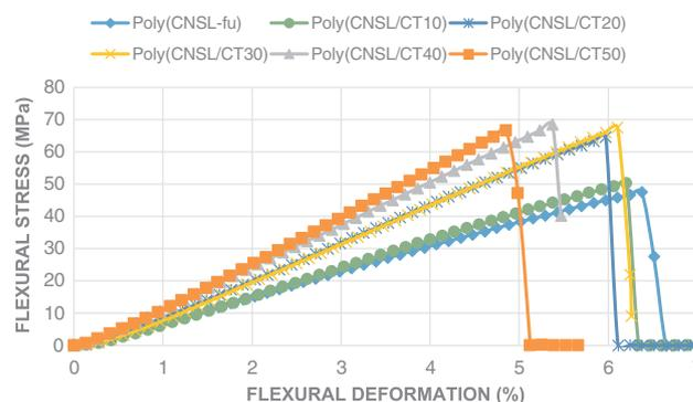
Fig. 5. Stress-strain curves obtained from 3-point bending of polybenzoxazines.
