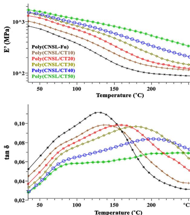
Fig. 6. DMA analyses of CT-fu/CNSL-fu copolymers.
