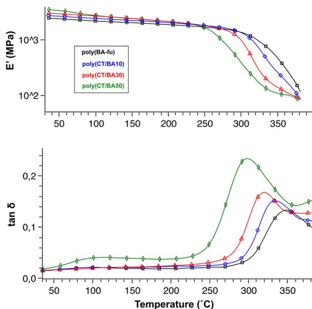
**Figure 6.** DMA curves of poly(BA-fu), poly(CT/BA10), poly(CT/BA30), and poly(CT/BA50).
