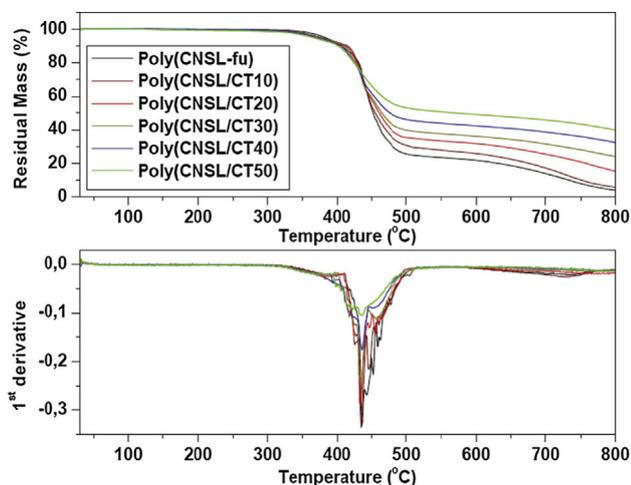
Fig. 4. TGA thermograms of (co)polybenzoxazines.
