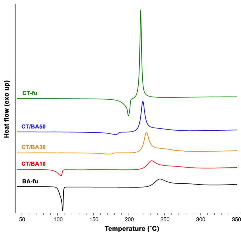
Figure 4. DSC curves of CT-fu, BA-fu, and different resins compositions (CT-fu/BA-fu).
