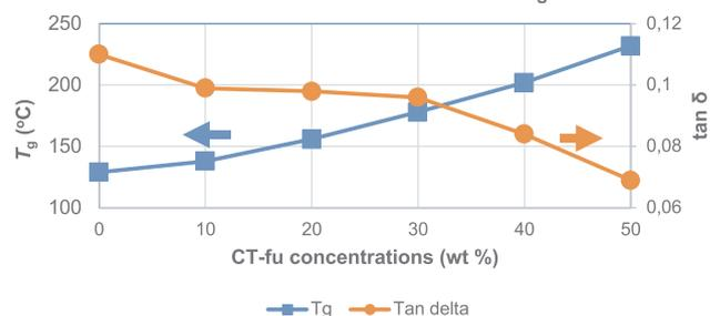
Fig. 8. Correlation of CT-fu/CNSL-fu concentration with  $\alpha$  transitions of the (co)polybenzoxazines.
