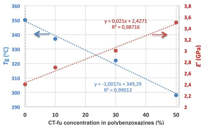
**Figure 7.** Linear correlations of  $T_g$  and  $E'$  with CT-fu concentrations.
