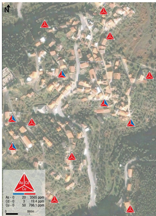
Fig. 5. Cartography of road dust contents for As, Cd and Cu (Google Earth image modified).
