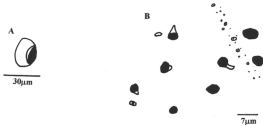
Figure 15. (A) Rounded solid of dolomite with a black portion of probably hydrocarbon and associated aqueous portion. (B) Inclusions with hydrocarbon and aqueous appendices. A little trail of aqueous inclusions and the occurrence of monophasic and biphasic inclusions apparently associated with inclusions with hydrocarbon.
