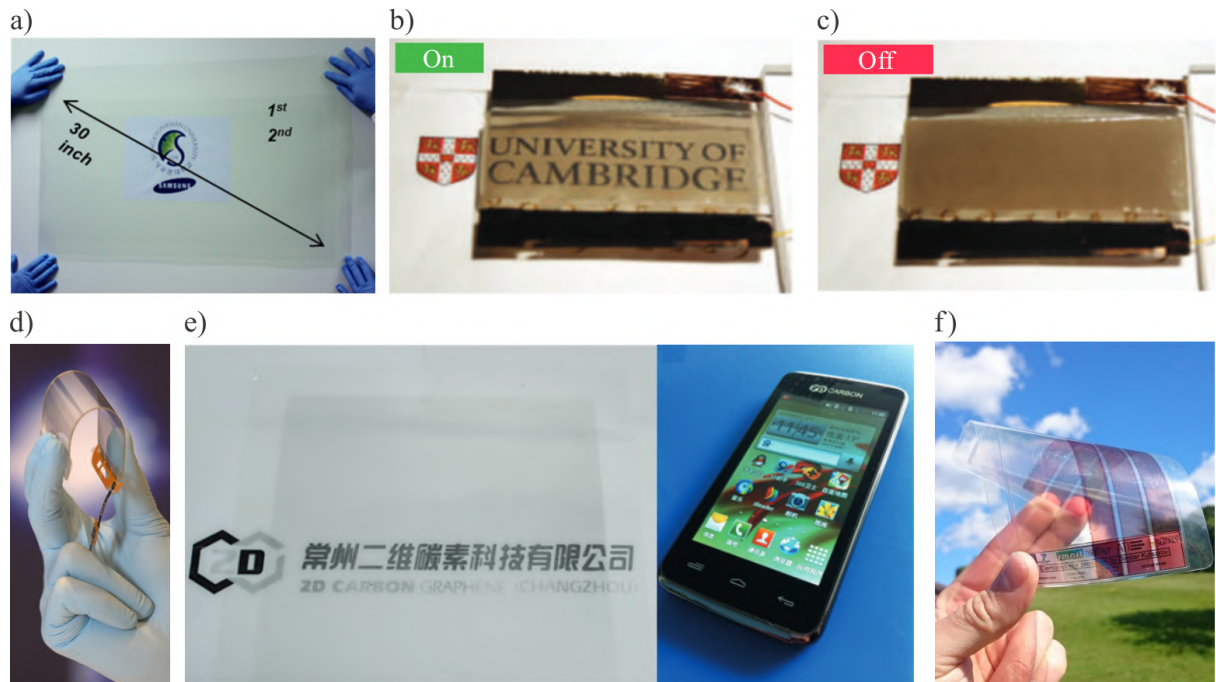
Figure 22: (a) Graphene-based display. A transparent smart window that can displaying information, when it is turn on, (b) or not (c), when is off. (d) Illustration of a thin graphene display emphasizing its flexibility. (e) Another example of a thin graphene-based conductive display (touch screen display) produced by the company 2D Carbon Tech (left) and its use as a prototype of smartphone display (right). (f) Illustration of a flexible photovoltaic cell modules. Adapted from Refs. [18, 26–29]
