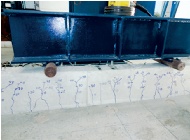
A VB-R beam in the collapse
