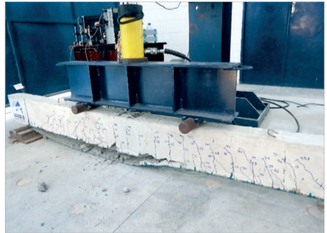
B VB-2 beam in the collapse
