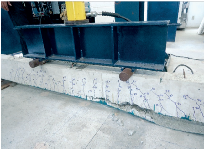
C VB-3 beam in the collapse
