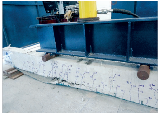
D VB-4 beam in the collapse
