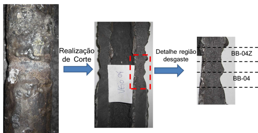
Figure 7. SEN images: (left) SEN after continuous casting; (centre) after cutting the SEN; (right) regions of the SEN for which different mould powders were used.
