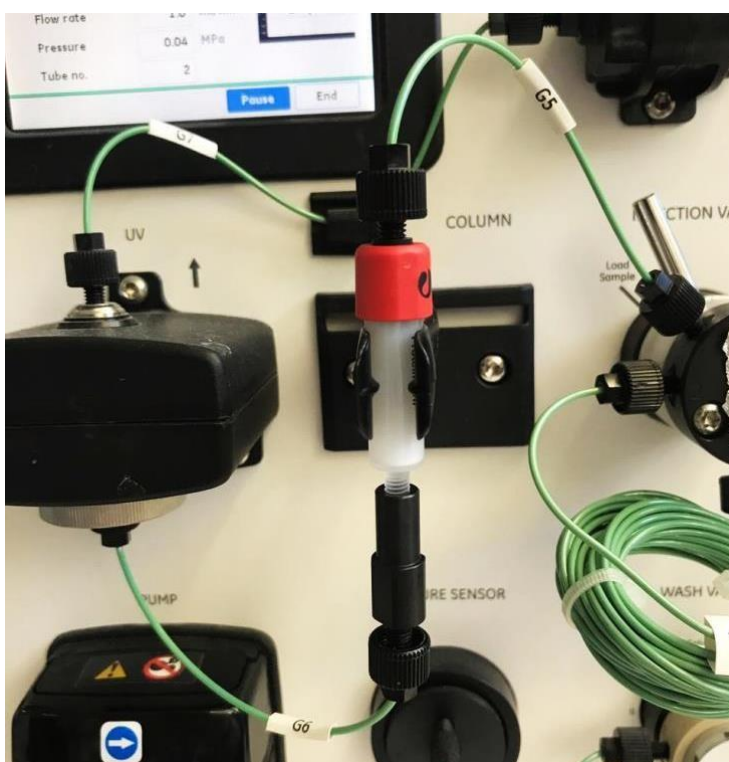
Figura 5 – Coluna HiTrap® Protein A acoplada no ÄKTA Start Protein Purification System
