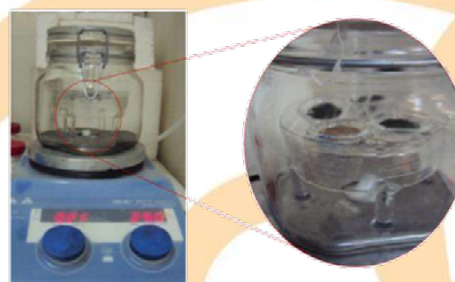
Fig. 2. Static system used in the batch adsorption studies.
