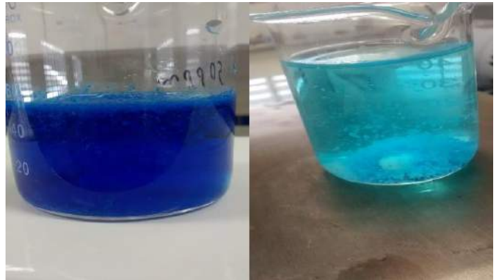
Figure 2. Effluent contaminated by MB (left) and after the ionic flocculation (right).
