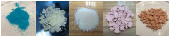
Fig.1. Photographs of synthesized MOPS powders: Cu BTC, Al BTC, Al BDC, Fe BTC, and Fe BDC, in the order of pictures.
