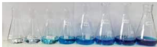
Fig. 9. Adsorption tests of methylene blue at different concentrations.
