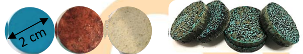
Fig.2. Photographs of shaped MOPS samples: Cu-BTC, Fe-BDC, Al-BTC, and the Cu-BTC/AC-6T composite, in the order of pictures.
