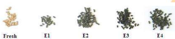
Fig. 5. Visual appearance of the molecular sieve AW500 fresh and deactivated.
