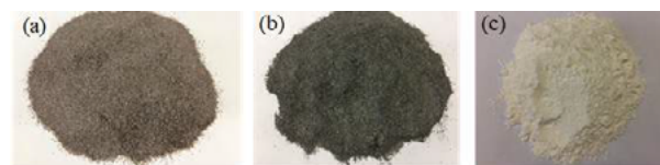
Fig. 3. Adsorbent materials produced: in natura (a), after pyrolysis (b) and after calcination (c).
