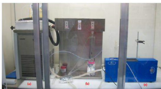
Fig. 3. Experimental set-up used in the dynamic adsorption studies. (a) Mercury saturator, (b) fixed-bed reactor, and (c) mercury analyzer.
