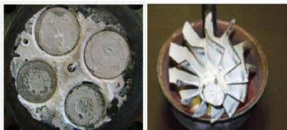
Fig. 2. Engine components damaged by siloxanes
