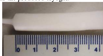
Fig. 1. Digital photograph of the polyacrylamide and chitosan cryogel synthesized.
