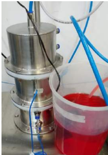
Fig. 1. Apparatus for adsorption by circulating percolation; wheat bran packed at central module.
