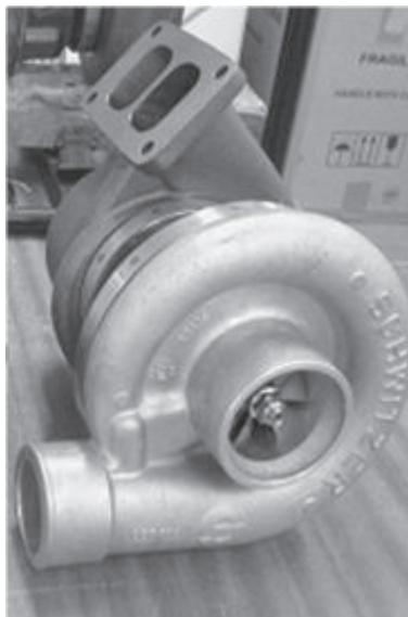
Figura 1: Turbocompressor 4LGZ
