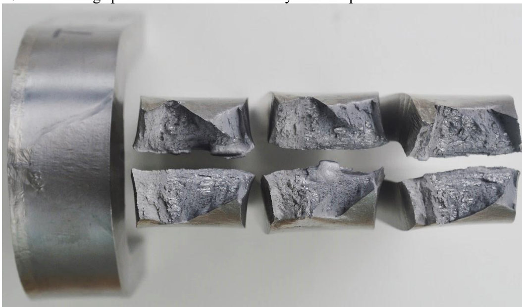
Figure 7-22. Bending specimens after the test. Only one sample did not break.
