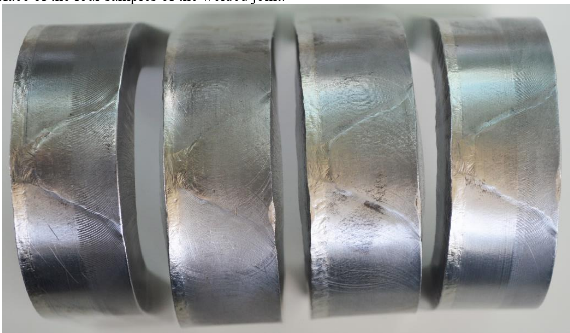
Figure 8-15. Bending specimens after the test. No samples showed any defects on the bending surface of the four samples of the welded joint.
