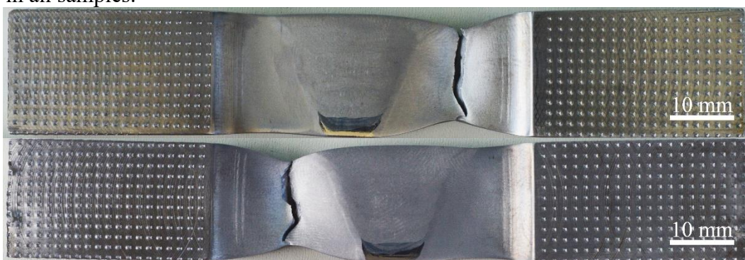
Figure 9-17. Transverse tensile test samples after the test. The fracture occurred in the base metal in all samples.
