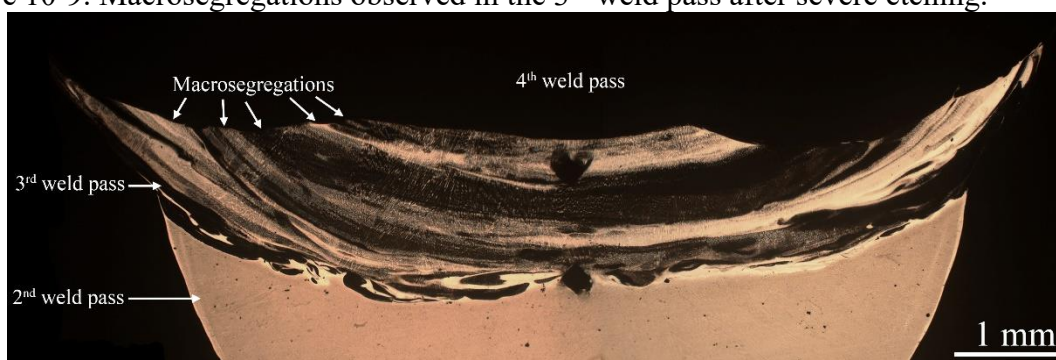
Figure 10-9. Macrosegregations observed in the 3 rd weld pass after severe etching.
