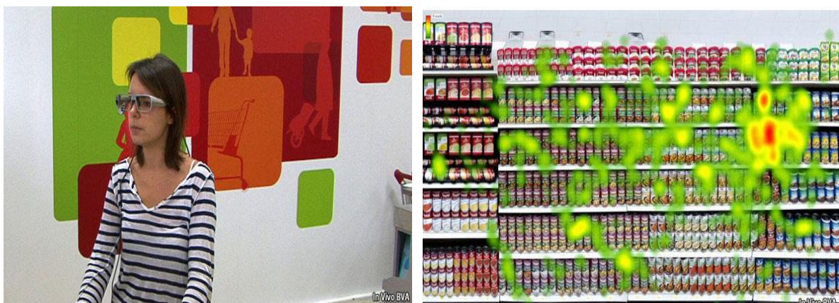
Figure 4 – (A) Woman wearing a mobile eye-tracker. (B) Heat map generated from looking at items in a supermarket (red areas represent more fixations)
