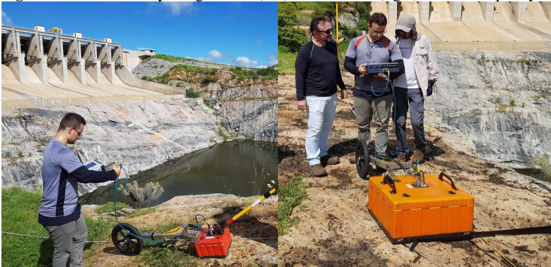
Figure 4.10 - GPR survey using the 200 (left) and 400MHz (right) antenna frequency
