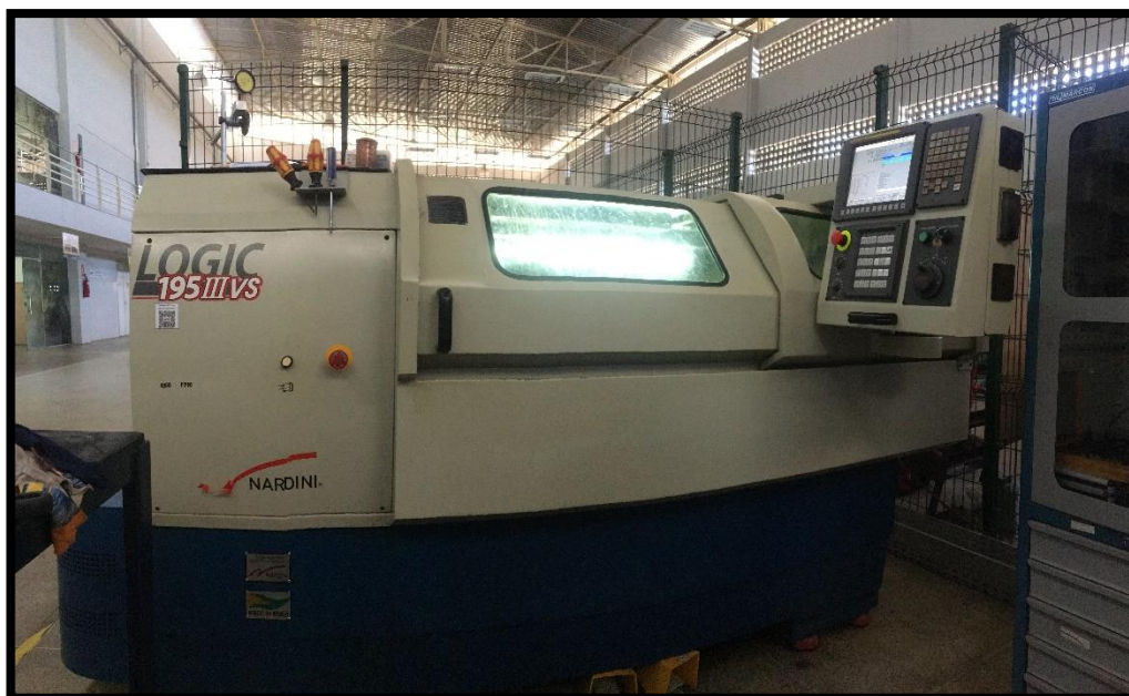
Figura 4.1: Torno Nardini LOGIC 195 III VS.
