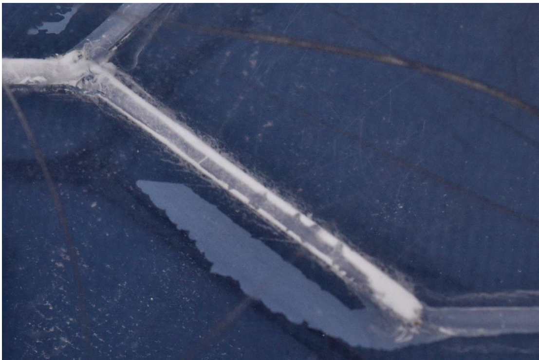
Figure 23 – Photograph of the mineral scales inside the acrylic chip
