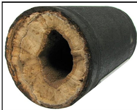
Figure 3 - Calcium carbonate scale in pipe
