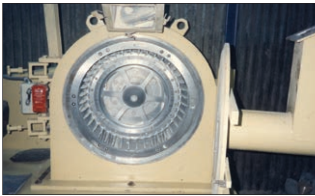
This view of a pulverizer shows its high-speed rotor.
