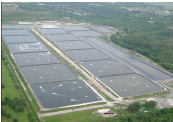
This intensive inland shrimp farm uses lined ponds, heavy aeration, water treatment, and recirculation. Photo courtesy of Oceanboy Farms, Florida, USA.
