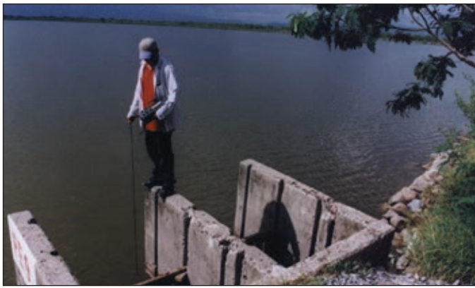
Monitoring of dissolved oxygen is a requirement of some regional use permits.
