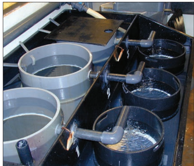
In this egg-hatching and nauplii-rinsing apparatus, the collector at top has a black cover with a hole to attract nauplii to the light for transfer in flowing sea water to the nauplii collection vessel. Photo courtesy of Unima.
