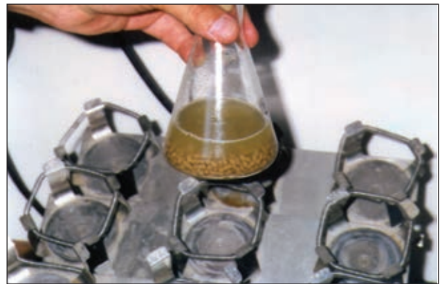
Water stability tests are ideally based on standardized immersion, agitation, and drying techniques.
