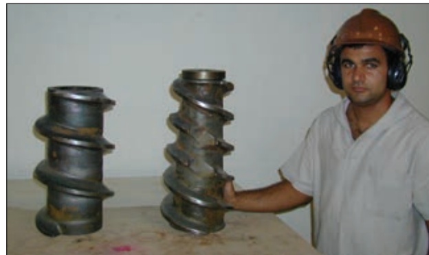
The screw sections in extruders are designed with variable pitch and depth to apply mechanical energy to cook the moist meal through heat, pressure, and shear.
