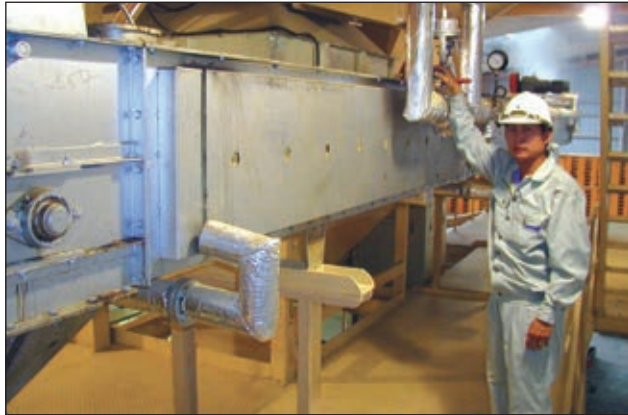
This postpellet conditioner uses a moving belt within a horizontal steam chamber.
