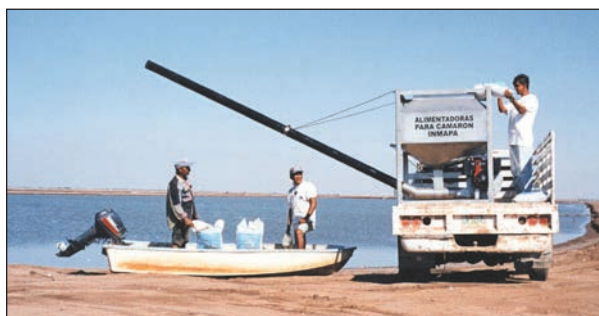
Many bigger farms distribute large quantities of feed from boats or vehicles with mechanical blowers.
