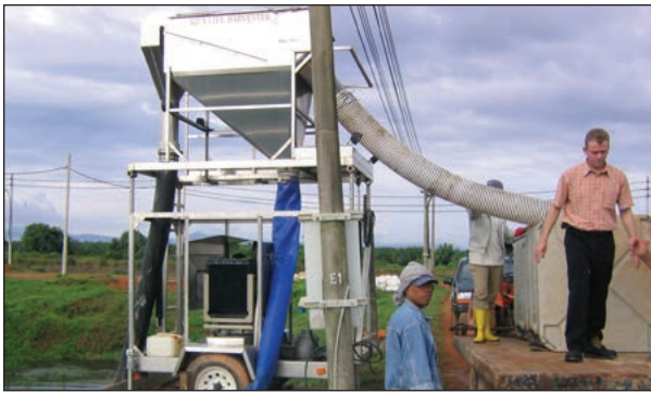
Harvesting with a shrimp pump. Such new approaches require specialized equipment, training, and investment.
