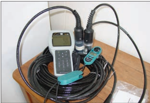
Water quality probes can be attached to long cables for monitoring parameters at depth in estuaries.
