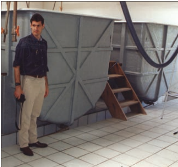
According to the survey, smaller tanks like the 10-cubic-meter fibreglass units above are gaining popularity over large rectangular concrete tanks.
