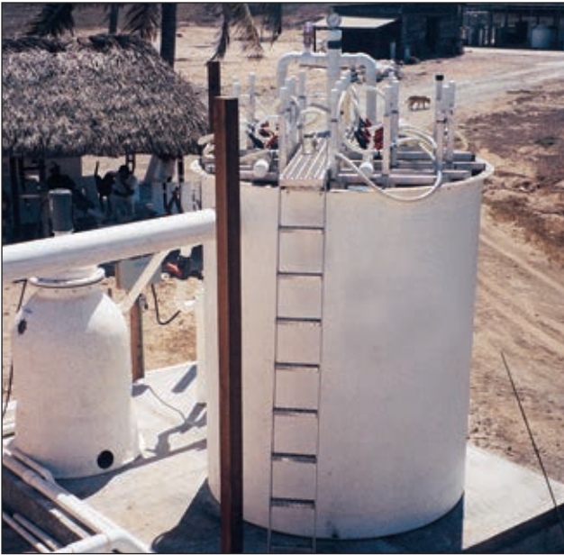
Fluidized-bed biofilter installed in a shrimp maturation system. Photo courtesy of Aquaneering.
