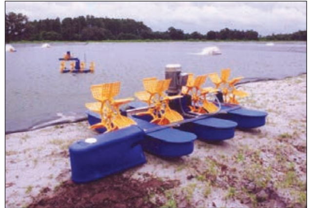
Paddlewheel aerators mechanically splash water into the air to cause oxygenation.
