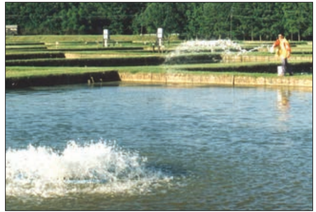
Vertical pump sprayers consist of a motor and impeller that jets water into the air to aerate pond water.
