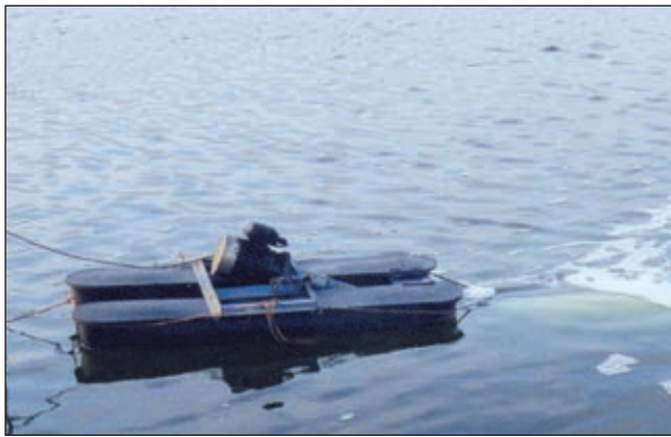
Propeller-aspirator-pump aerators have a spinning impeller and a hollow shaft that draws air from the surface and breaks it into fine bubbles in the pond.
