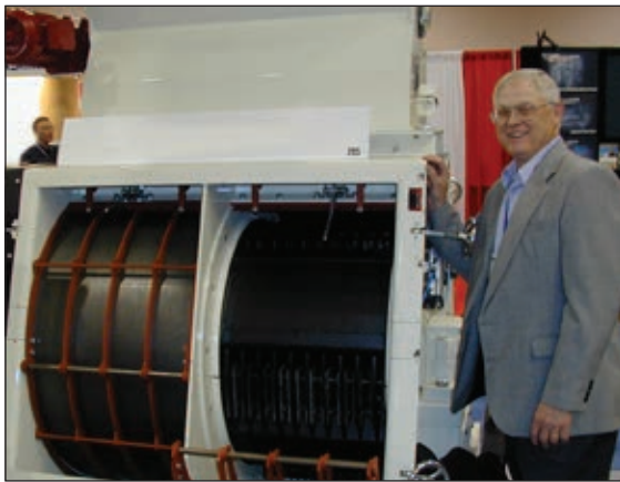
This open hammermill shows the screen installed on the left, and removed on the right to expose articulating hammers.
