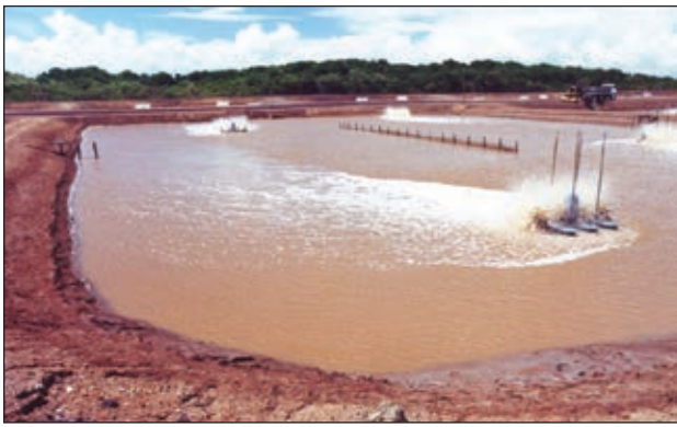
Paddlewheel aerators can be arranged to wash out pond corners and circulate water to move wastes to the center for easier removal.
