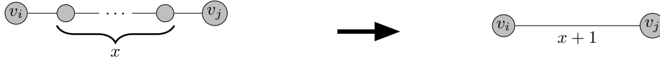
Figure 4: A weighted edge on the right and the real structure on the left.
