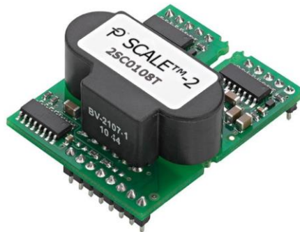
Figure 4.8 – Photo of the driver “Dual-Channel SCALE™-2+ 2SC0108T-17” from PowerIntegrations®.
