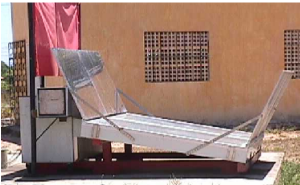
Fig. 1 Solar cooker with temporary heat storage tank and a baking oven.
