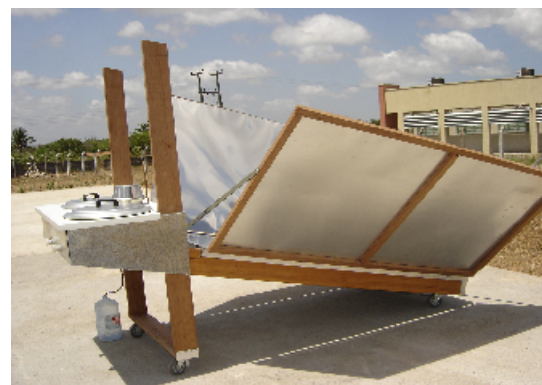
Fig. 2 Solar cooker manufactured in Brazil. In the photograph, the top reflector had not been yet installed
