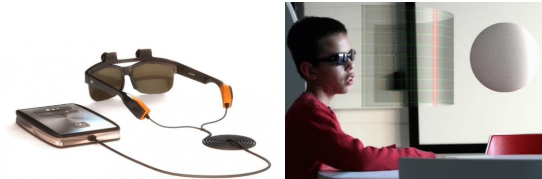
Figure 12. EyeSynth equipment and scheme of tracking mode, where the glasses only capture the central, front view. The user has to sweep left and right, in a similar way as when using a cane.
