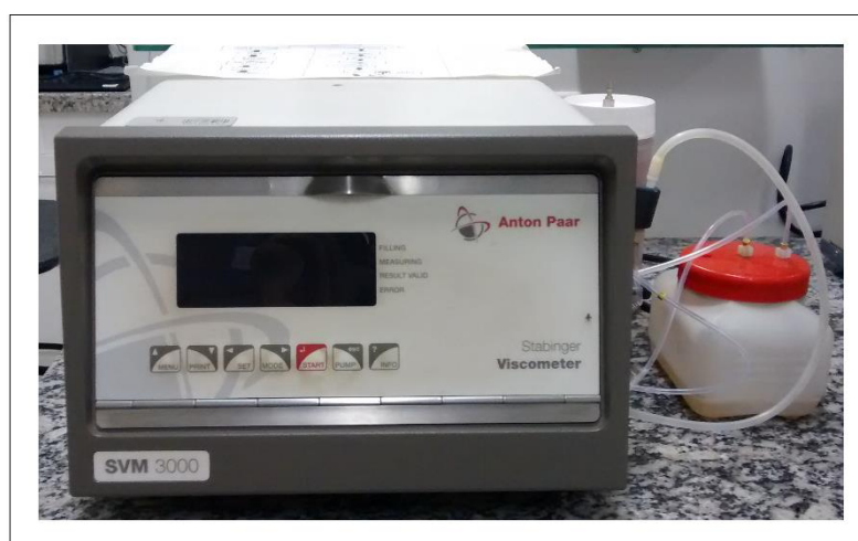
Figura 3.5 - Viscodensímetro digital Anton Paar SVM 3000-Stabinger
