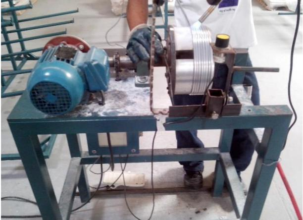
A photograph showing a person in a white shirt and blue gloves operating a blue motorized machine. The machine is mounted on a blue metal stand and is used to form a helical coil of metal tubing. The worker is positioned behind the machine, and the coil is visible on the right side of the machine. |
