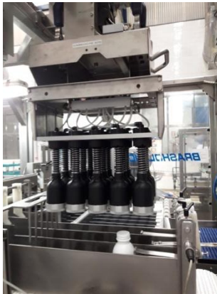
Figura 5 – Cabeçote de Tulipas – Pick & Place
