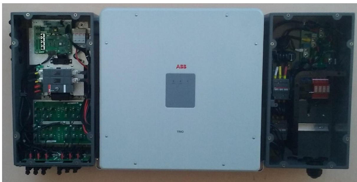
Figura 4 – Inversor ABB TRIO-50.0-TL-OUTD – 50 kW.
